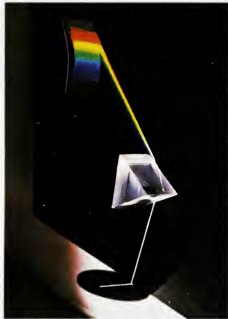
Spectrum of white light by (above) a prism and (below) a diffraction grating. With a prism, the red end of the spectrum is more compressed than the violet end.
